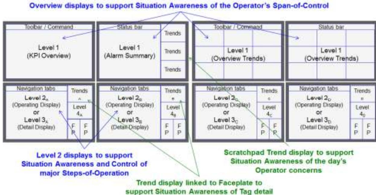
**Figure 2** A conceptual illustration of an 'ASM-compliant' console operator HMI, and the simultaneous support for proactive operator situation awareness from 'big picture' to tag detail (in this case, with a drill-down navigation approach)
